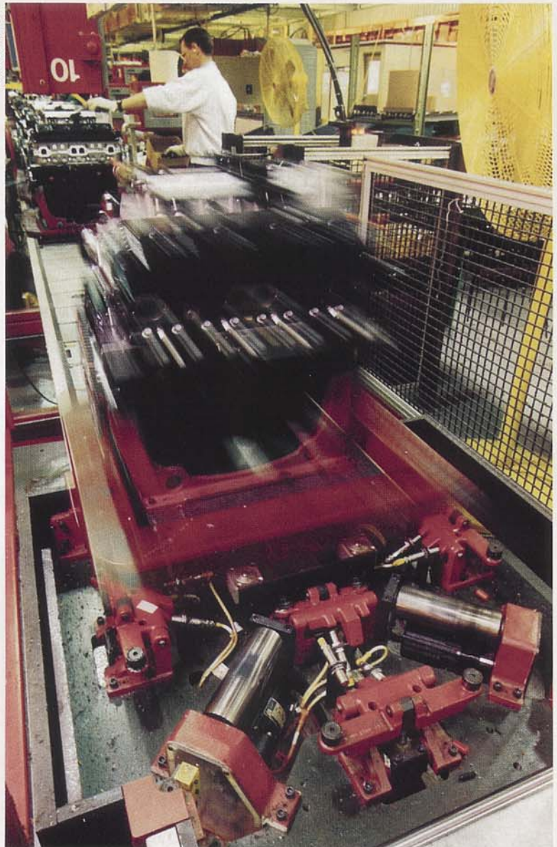
SmartConveyor's motors help transport an engine in GM's Flint, Mich., plant.
